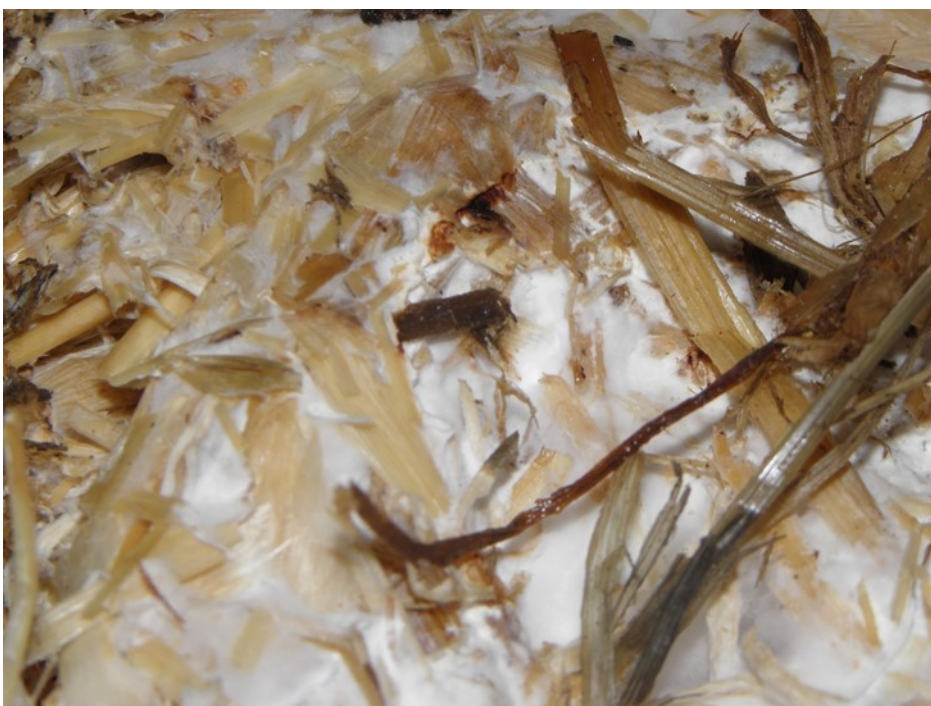
Figure 13. White nutrient produced from plant material for consumption by the bacteria. The plant material in the photo is removed by screening before delivery to the plant.
