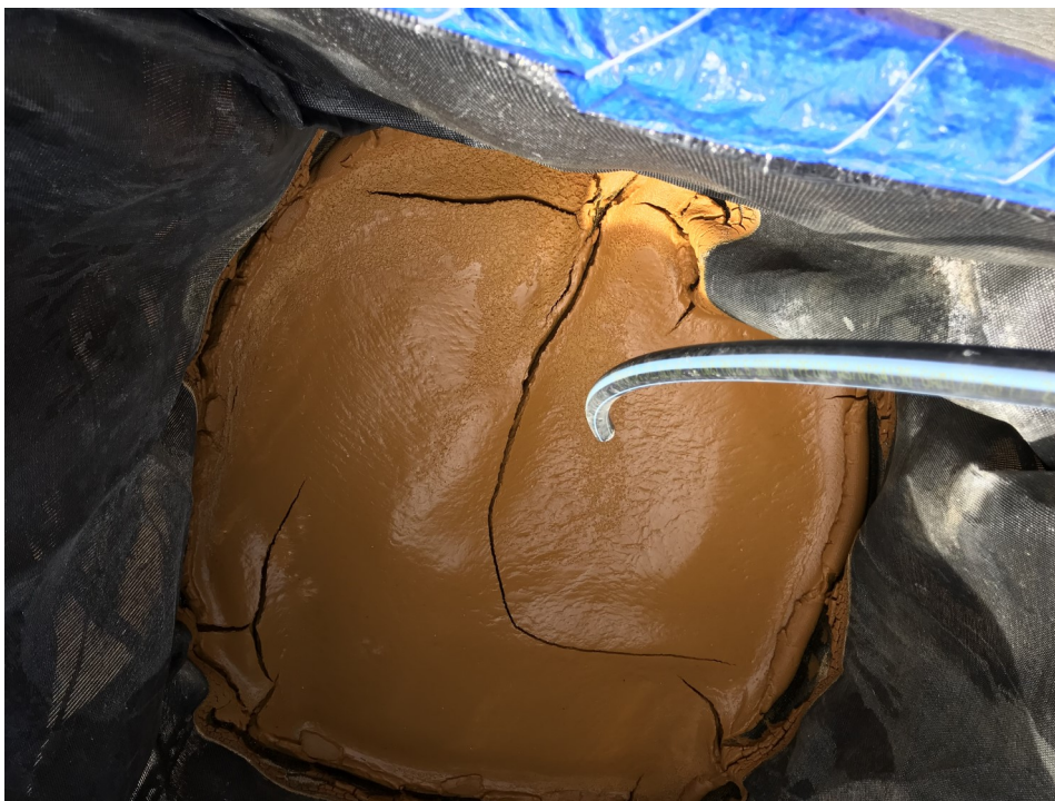
Figure 3. Metals in an operating metal oxide geobag
