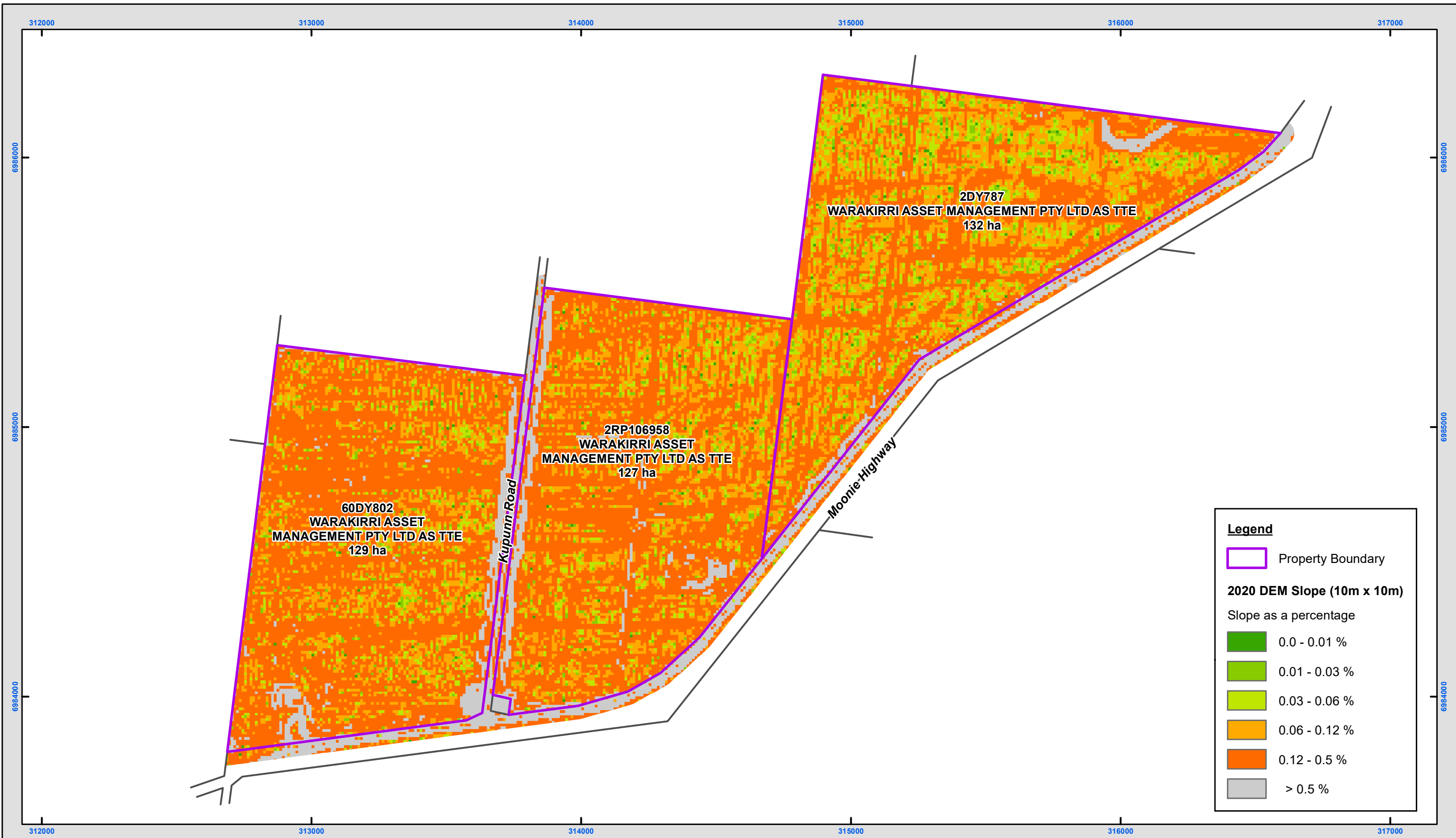
Figure 6 : Slope Analysis (10m x 10m squares) of 2020 DEM : Lots on Plans 60DY802, 2RP106958 & 2DY787
