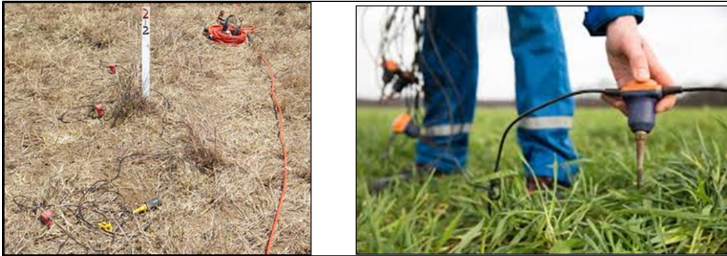
Figure 7 Geophone and Geophone Placement (type shown are connected by cables, most likely the survey will deploy 'cableless' geophones)
