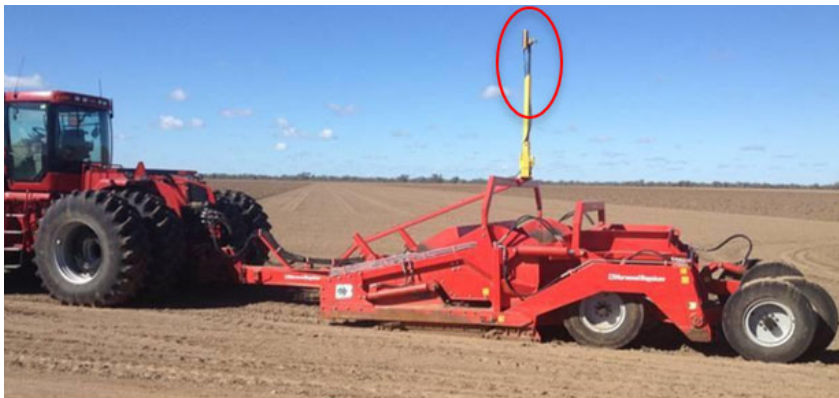
Figure 9: Laser bucket operating in the field with the laser receiver circled (source Justheavyequipment.com.au)
