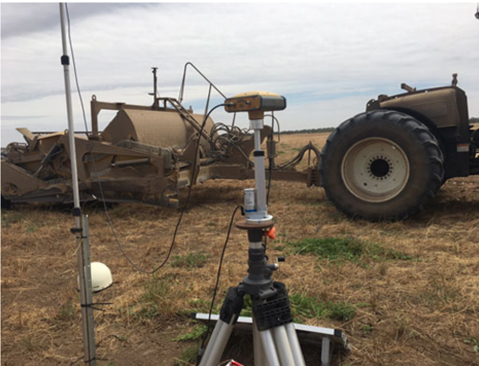
Figure 27: The Toomey linear actuator fitted to a GNSS base station (Source Toomey)
