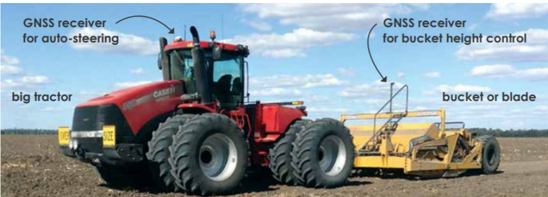
Figure 11: Single receiver GNSS land levelling components (source Tim Neale), and dual antennae options below (Source BMS lasersat)
