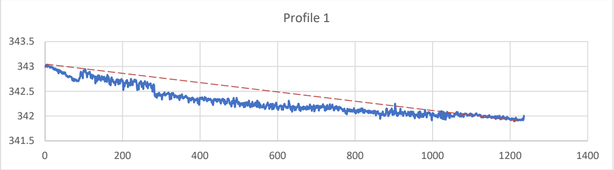
Figure 2: Twenty-six elevation profiles of randomly selected paddocks (X and Y Axis are all in metres – Y = vertical, X = distance from start point). The red dashed line represents average slope drawn across each field.
