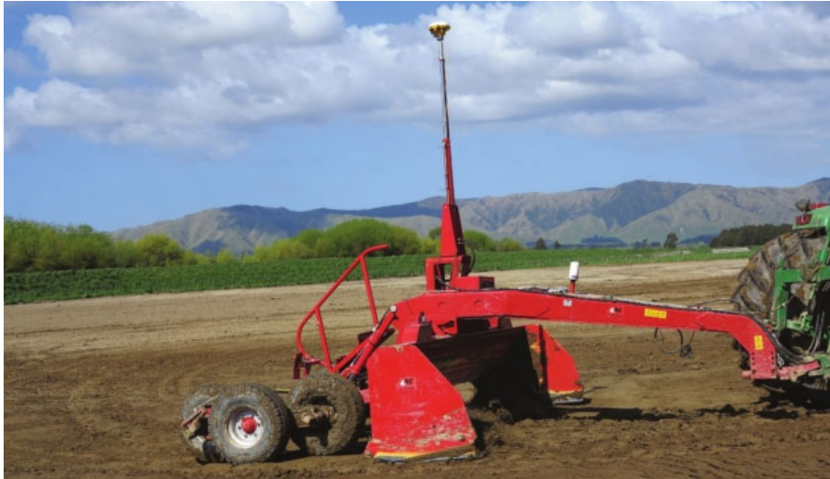
Figure 12: levelling blade and Pulldozer style levelling options (source Optisurface top, and Pulldozer bottom – source Bridgeview manufacturing)
