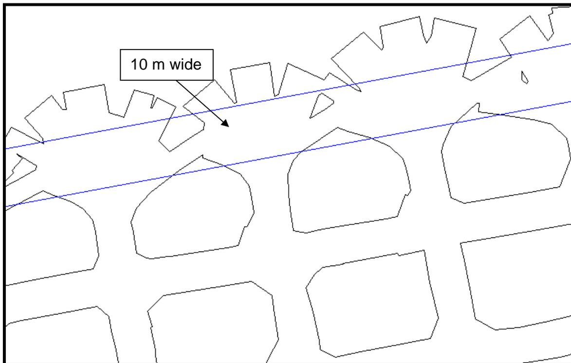
**Figure 27. Comparison of Bell Out and Standard Pillars**
