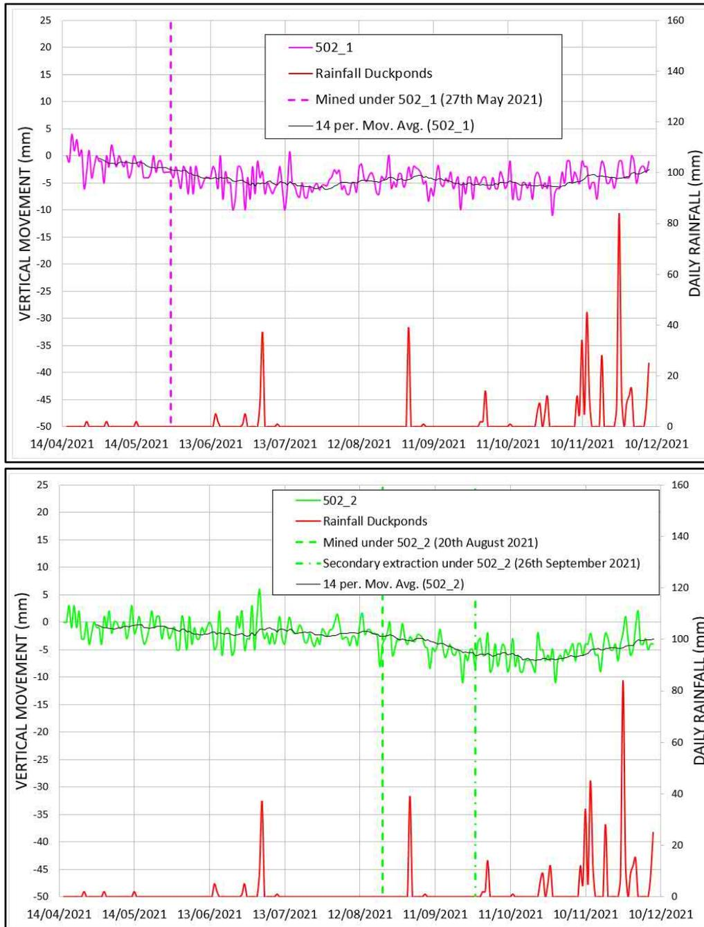
**Figure 17. Subsidence Monitoring above 500 Mains and 502 Panel**
