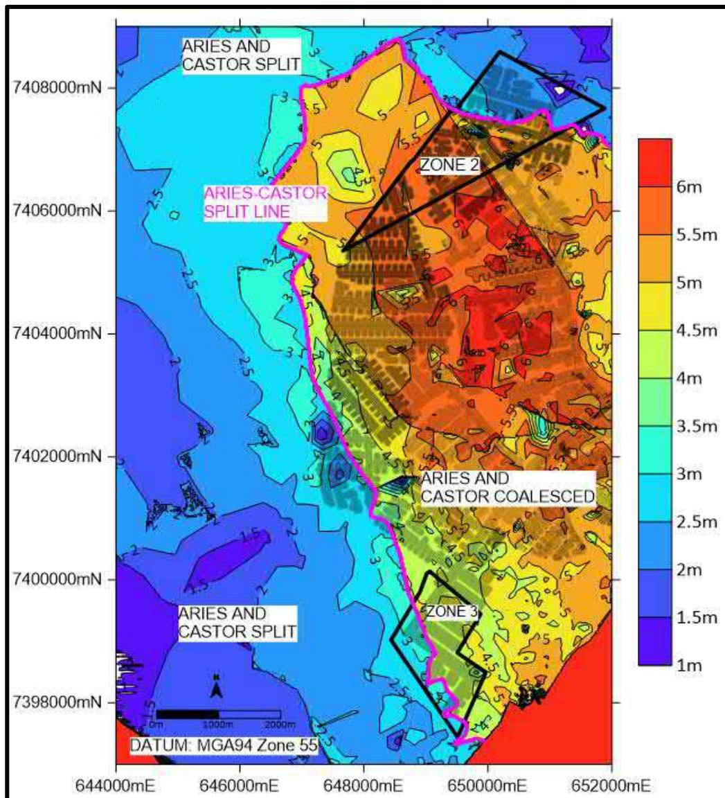
**Figure 11. Working Section Thickness**
