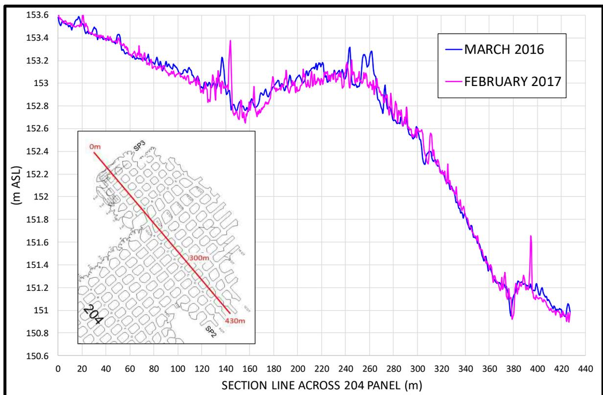
**Figure 20. Section Line above 204 Panel**
