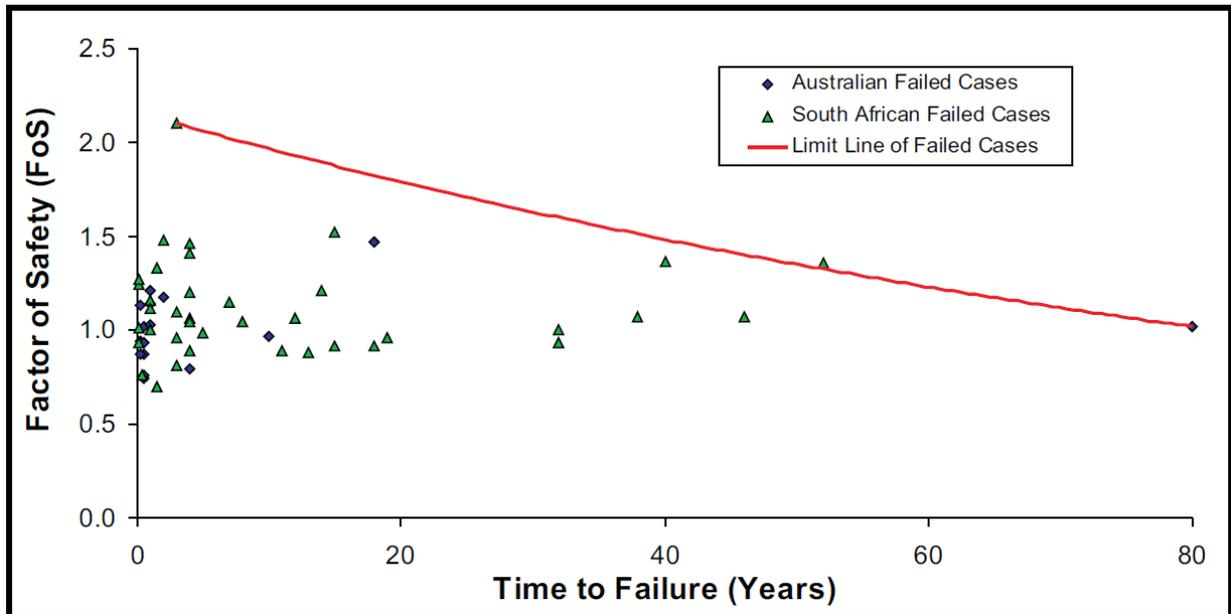
**Figure 36. Factor of Safety versus Time to Failure**
