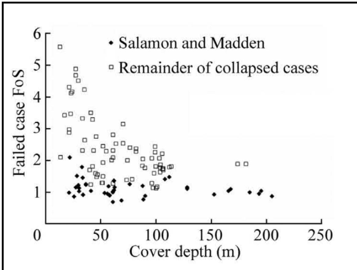
**Figure 37. Factor of Safety vs Depth of Cover**
