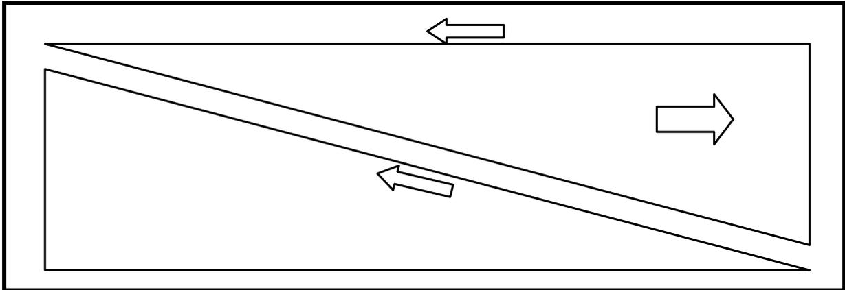
**Figure 33. Kinematic Failure of Wedges**
