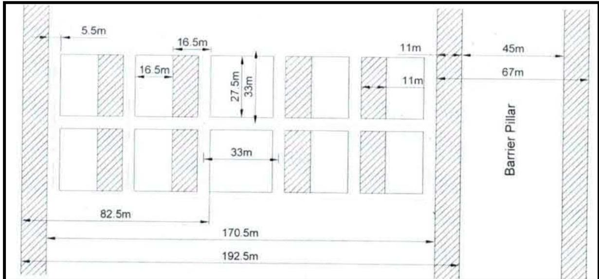
**Figure 22. Bord and Pillar Layout – Clarence Mine**
