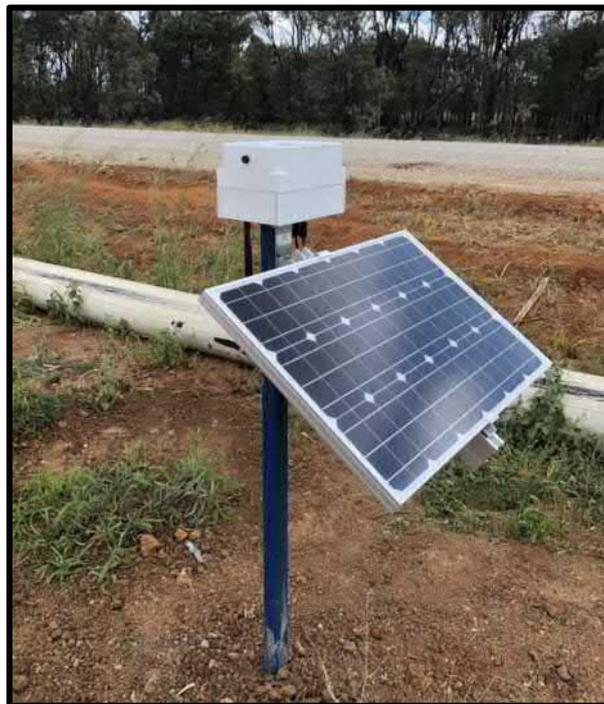
**Figure 14. Fixed GPS Monitoring Station**
