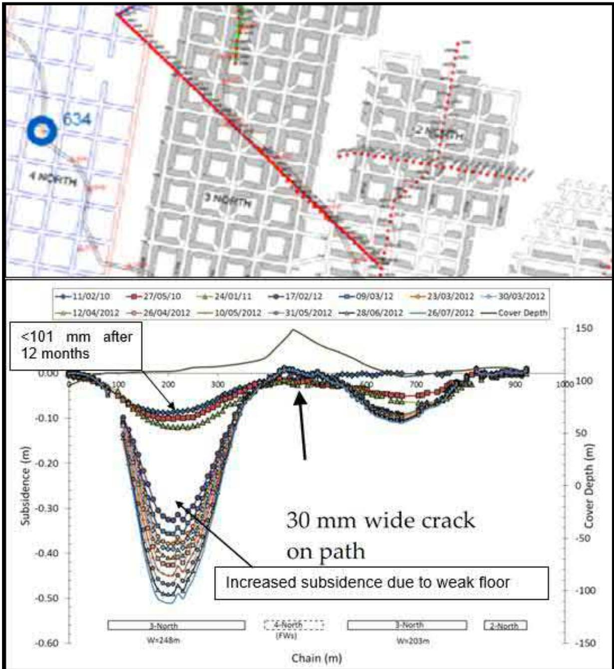
**Figure 23. Subsidence over 3 North Panel at Tasman**
