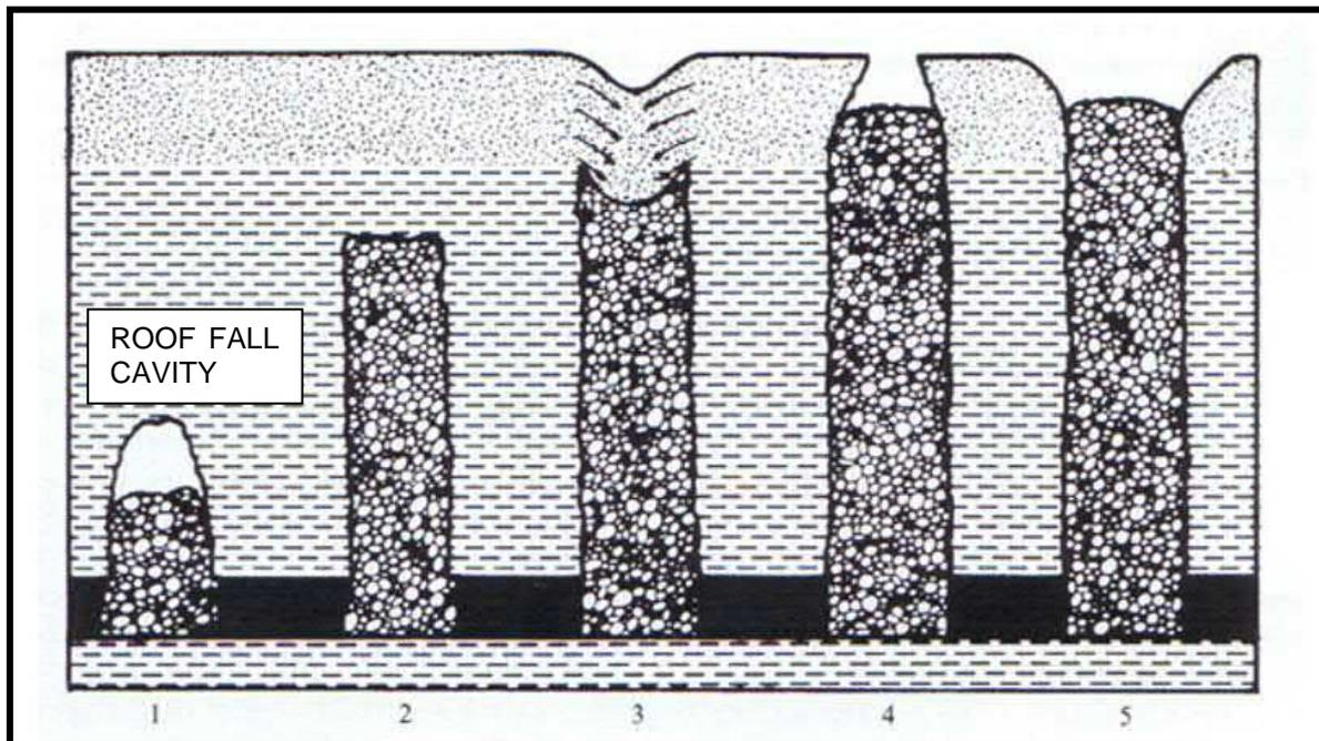
**Figure 39. Illustration of Suggested Sinkhole Development Mechanism (Whittaker and Reddish, 1989).**
