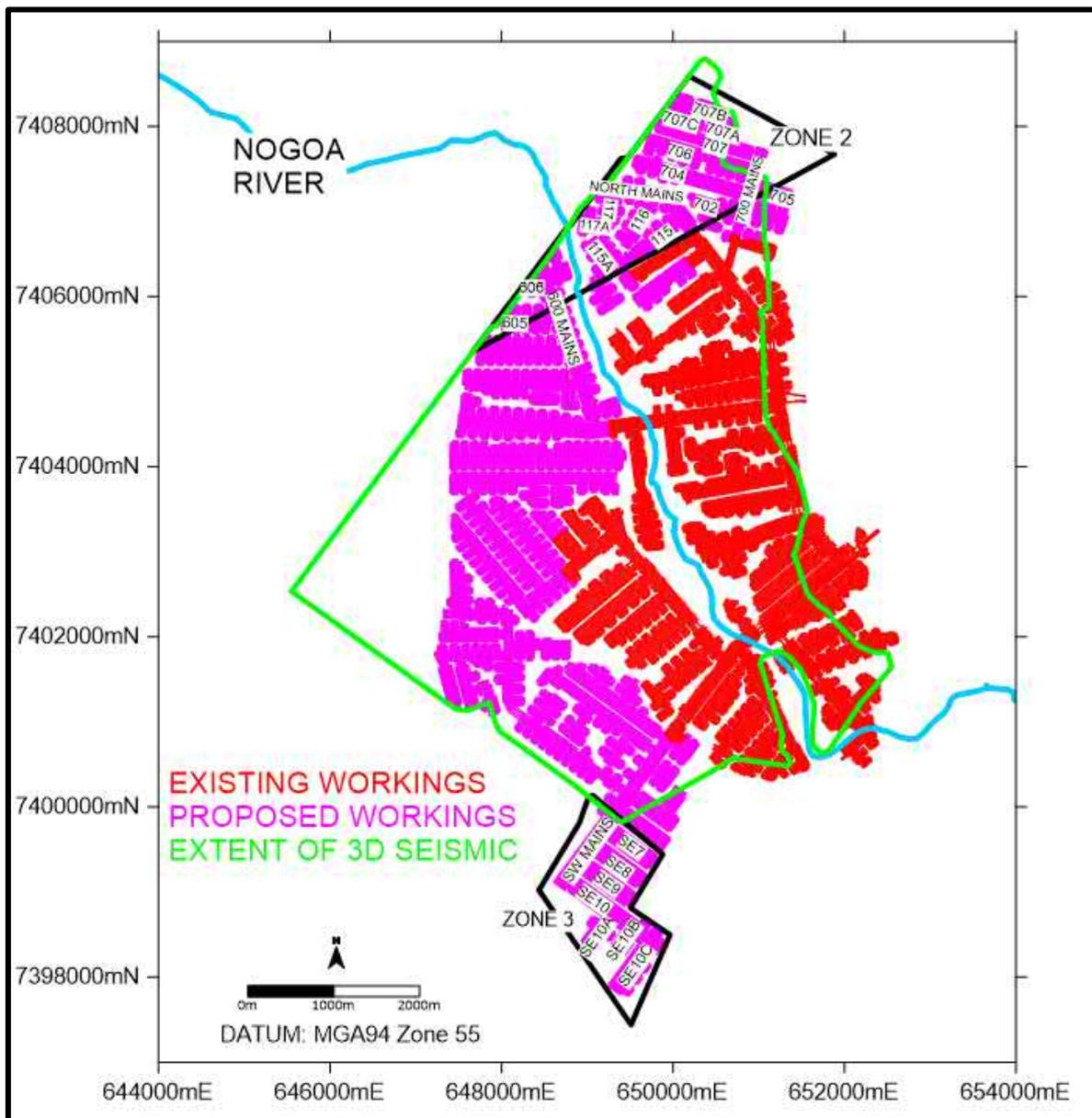
**Figure 8. Bord and Pillar Panel Nomenclature and Outline of 3D Seismic**
